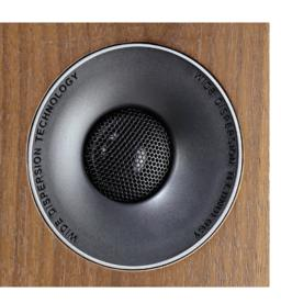
The 28mm aluminium dome tweeter is larger than most (25mm) and is aided by a shallow waveguide to give smooth output up to 20kHz.
